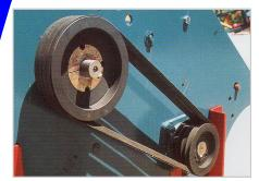
Belt drives lessen the shock loads which mulchers have to endure. Consisting of either 3 or 4 belts, depending on size, they are fitted using taper lock pulleys for ease of maintenance (pictured left).
