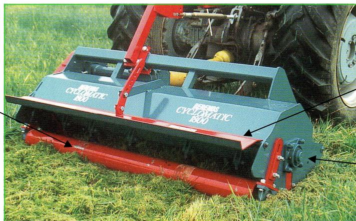
Adjustable back flap doubles as a scraper for the roller when in the mulching position.
