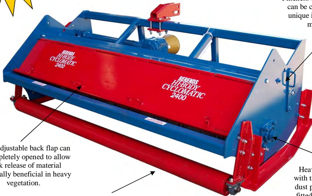
Fineness of mulching material can be controlled using the unique internal, adjustable mulching bar.
