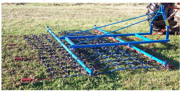
Before you connect the linkage frame to the harrows you need to connect the red drawbar chain to the tractor draw bar and take out the slack by pulling the harrows back or driving the tractor slightly forwards. This prevents the chain from dragging on the ground whilst providing some support to the main channel.
