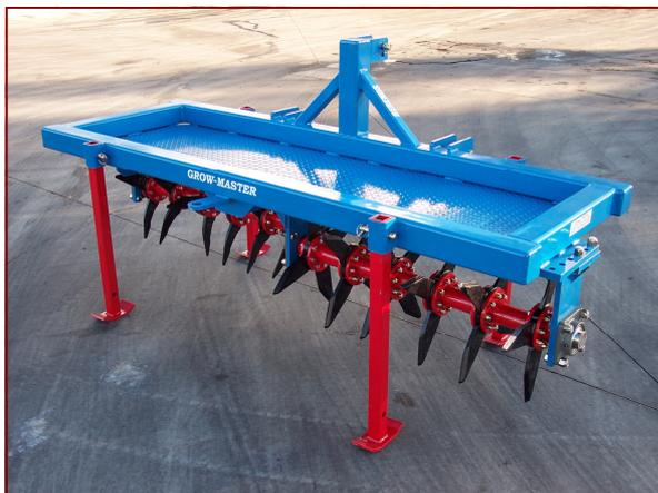
The **GROW-MASTER** is available in 2.0m, 2.4m, 2.8m and 3.2m working widths. Horsepower requirement is quite low with a minimum of only 35Hp required for the 2.0m unit.
